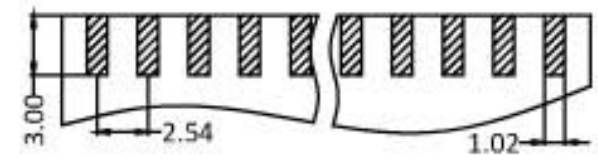
Recommended P.C.B Layout(TOP Side) (PCB BOARD TOLERANCE±0.05)
